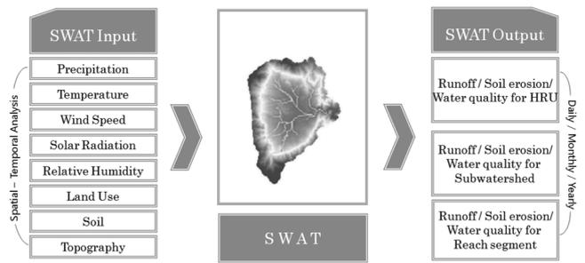
Fig. 4 Input and output data of the SWAT model
